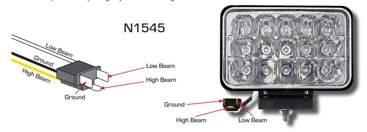
Determine the function of each wire coming from your vehicle's wiring harness (eg. ground, high beam and low beam). If what you find is different from the configuration in figure A or C, you will need to make necessary adjustments by either switching wire positions in the connection plug (wiring harness) or by using an adapter.
