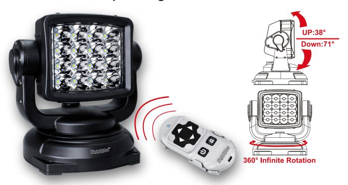
This light can fully rotate around its axis (360°) and tilt 110°. The beam is directed remotely with the help of a remote control unit, activating or deactivating the LED panel and two different motors, one for the tilting the other for the rotating movement.
