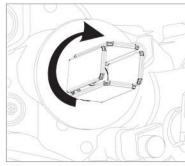
Turn clockwise until bulb is locked into place.
